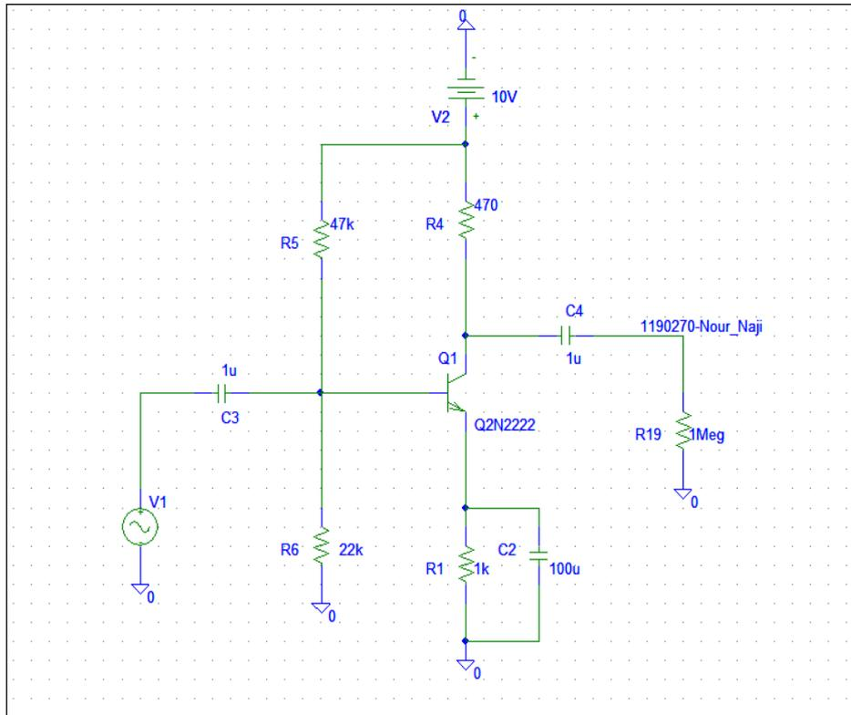
❖ DC bias and measure  $V_B$ ,  $V_C$ ,  $V_E$ ,  $I_C$  and  $I_B$ :
