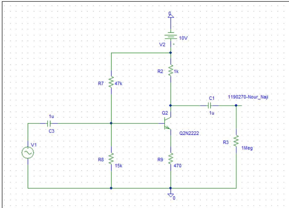
❖ DC bias and measure  $V_B$ ,  $V_C$ ,  $V_E$ ,  $I_C$  and  $I_B$ :
