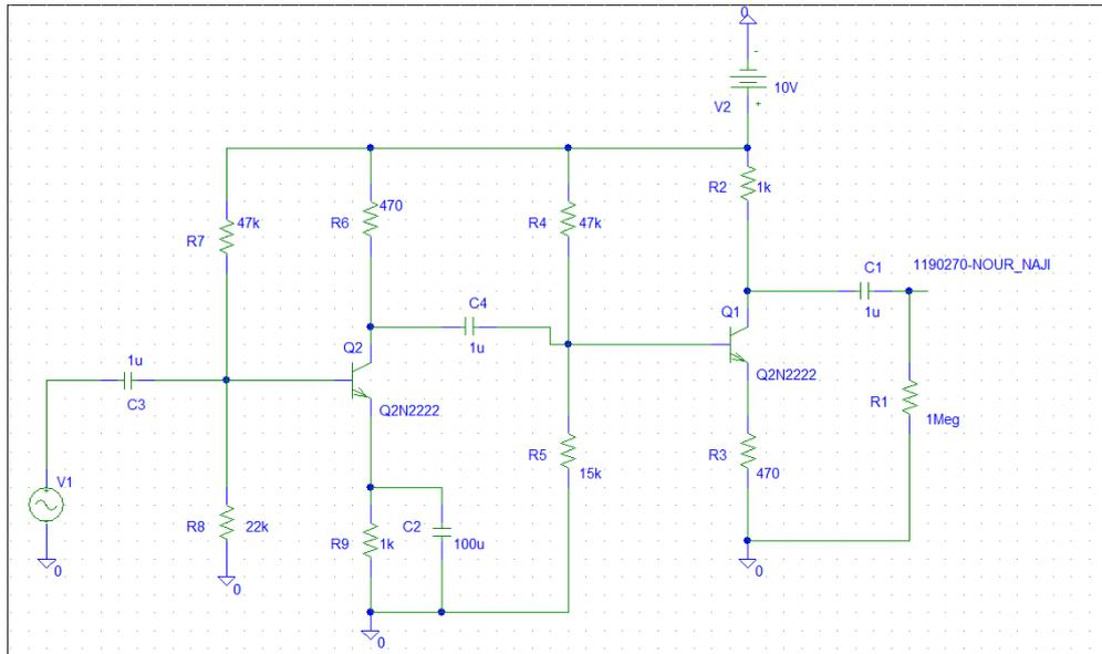
❖ DC bias and measure  $V_{B1}, V_{C1}, V_{E1}, I_{C1}$  and  $I_{B1}$  for first amplifier stage,  $V_{B2}, V_{C2}, V_{E2}, I_{C2}$  and  $I_{B2}$  for second amplifier stage:
